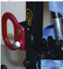
EZ Rider Bus Transport tie-down to secure chair while in transit.
