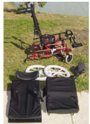
SAS8500 wheelchair with headrest, chest harness, flip-up and height adjustable armrests, multi-adjusted
