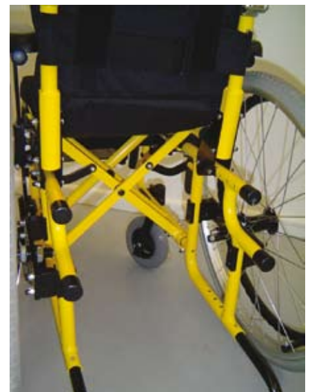
Double cross bars strengthen the frame.
