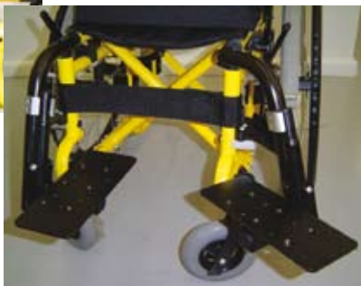
Swing-away footrests can adjust angle, depth and height.
