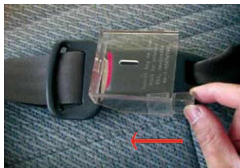
2. Insert Wedge-shape Spacer (can be broken into two pieces), slide along wall to take up loose space.
